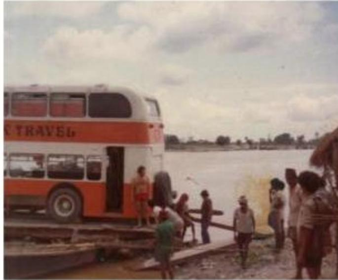
Grunt was manoeuvred onto the boat tearing up the overhang at the back of the bus. Blocks and rocks had to be placed under the rear wheels to keep the rear end off of the ground. Because when the rear end grounded the rear wheels lost traction and just spun free.
